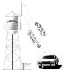
Because the transmitter and receiver are on at the same time, isolation must exist to keep the repeater's own transmitter from degrading the repeater receiver. If the repeater transmitter and receiver are not isolated well, the repeater's own transmitter *desensitizes* the repeater receiver. The problem is similar to being at a rock concert and not being able to hear the weak signal of a conversation over the much stronger signal of the band.
